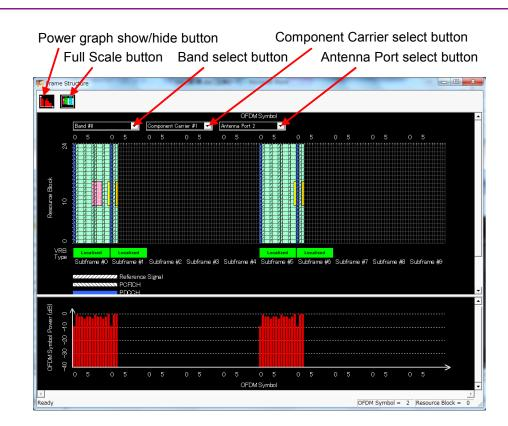
Figure 3.1.7-2 Frame Structure screen and power graph (LTE-Advanced)
