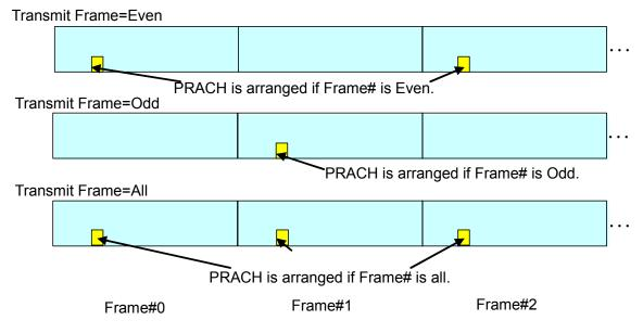
Figure 3.2-2 PRACH Frame Arrangement by Transmit Frame
