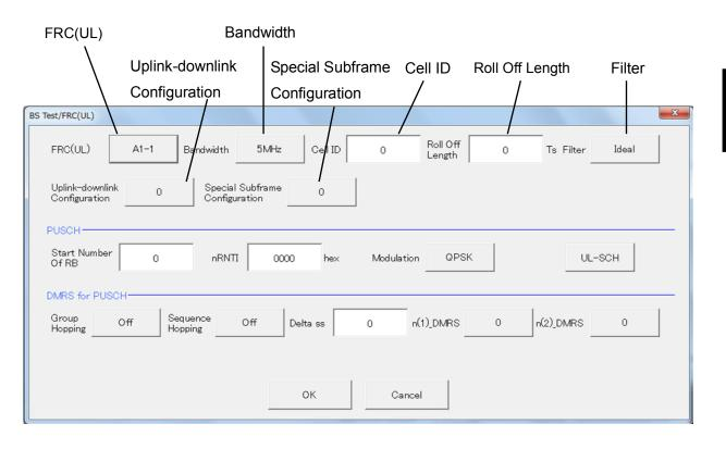
Figure 4.4.3.1-1 BS Test/FRC(UL) Common Parameter Setting Screen
